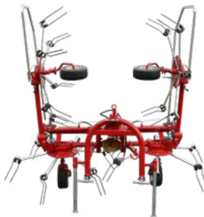
MINIMAL TRANSPORTATION FOOTPRINT POSSIBLE WITH 180° BASKET ROTATION
